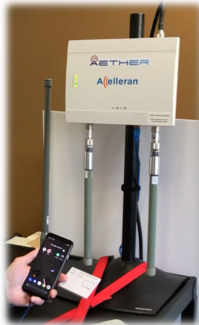
Small cells providing 4G/5G capacity and coverage serving real-life traffic for Internet access and edge applications
